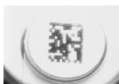
Washed out and Axial Distortion
