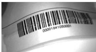
Figure 24 - Barcode Printed on Curved Surface Readable by Matrix 410N™ in spite of Image Optical Distortion
