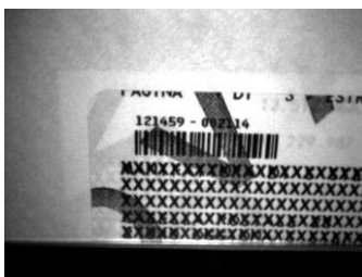
Figure 23 - Overprinted Barcode Readable by Matrix 410N™ also Through the Envelope Window Film
