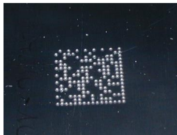
Figure 27 - Directly Marked Dot Matrix Code Characterized by Outstanding Separation Distance between Adjacent Code Elements
