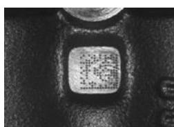
Dot Peening On Scratched Surface
